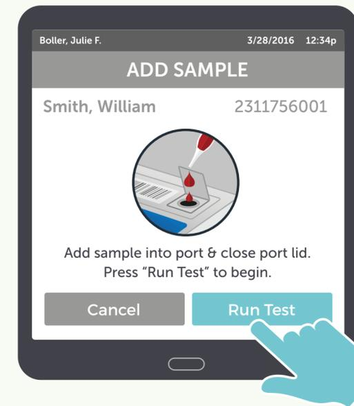
User prompted to expose port on cartridge, add sample, and run test
